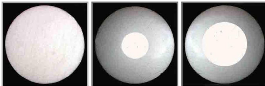
Figure 1 [Original Magnification: 200X]: The three materials tested here were (from left to right): Solid Nitinol wire, NiTi-DFT-10%Pt, and NiTi-DFT-30%Pt. A clean Nitinol to platinum interface, as shown, is an important characteristic of Nitinol composite material.
